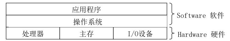
Layered view of a computer system 计算机系统的分层视图
